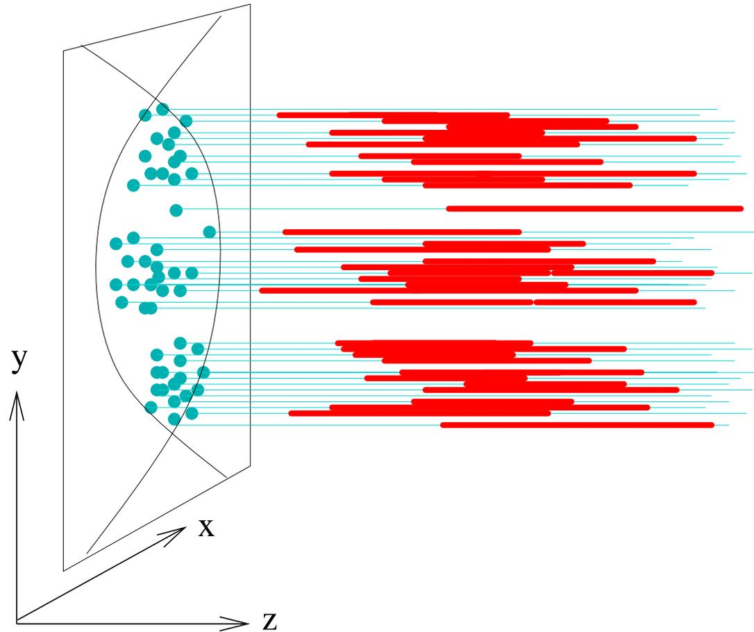
Projection of the positions of nucleon-nucleon scattering to the transverse  $(x, y)$  plane, which defines “possible transverse positions” of the flux tubes (thin lines).
