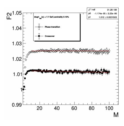
Fit the level of maximum with polinom of the first order: a+b x M b is of the order of 10-6
